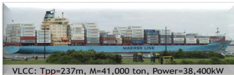
VLCC: Tpp=237m, M=41,000 ton, Power=38,400kW
