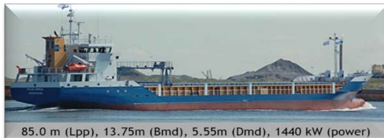
85.0 m (Lpp), 13.75m (Bmd), 5.55m (Dmd), 1440 kW (power)
