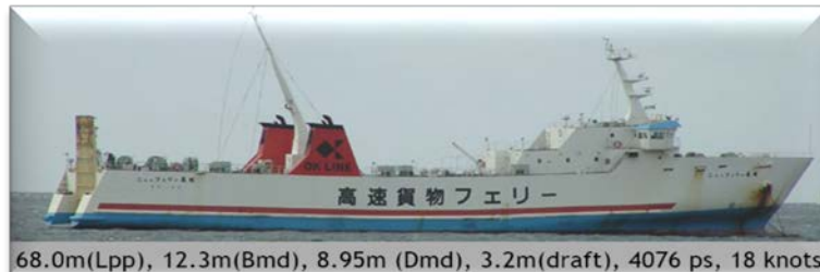
68.0m(Lpp), 12.3m(Bmd), 8.95m(Dmd), 3.2m(draft), 4076 ps, 18 knots
